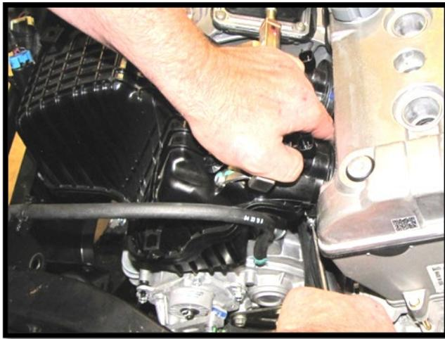
d. Loosen the hose clamp at the throttle inlet and pull the hose off. Then pull the intake manifold and fuel rail out and set aside for now.
