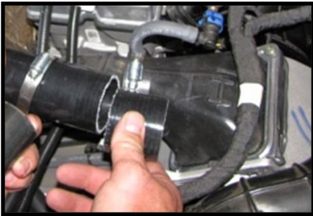
44. Next, slide the **SK-P-1506** (3" pipe) into the clutch outlet duct. Center it and slide the clutch exhaust hose on. Attach and tighten with two **HC36** hose clamps.
