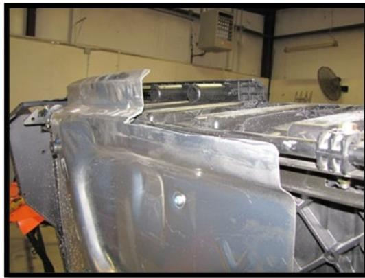
54. Find the bed plate **75L**. Center it on the bed using the large holes and where it meets the snorkels. Then trace the inside with a marker.
