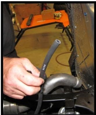
61. Insert a barbed fitting **BHF-14-ST** into the vent hose, followed by a bellow **VB01**. Use **11" zip ties** to secure the hose and bellow to the frame in a place it won't get damaged.
