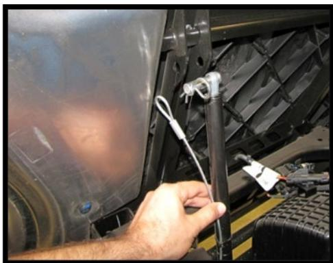
2. Remove the factory clutch outlet duct along with the metal mount bracket. You will reuse the metal mount bracket later with the new exhaust duct provided.
