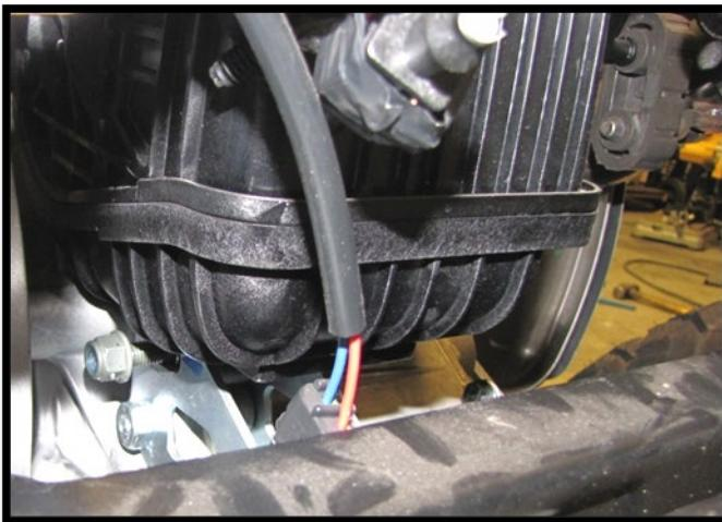
c. Reconnect the fuel line into the fuel rail.
