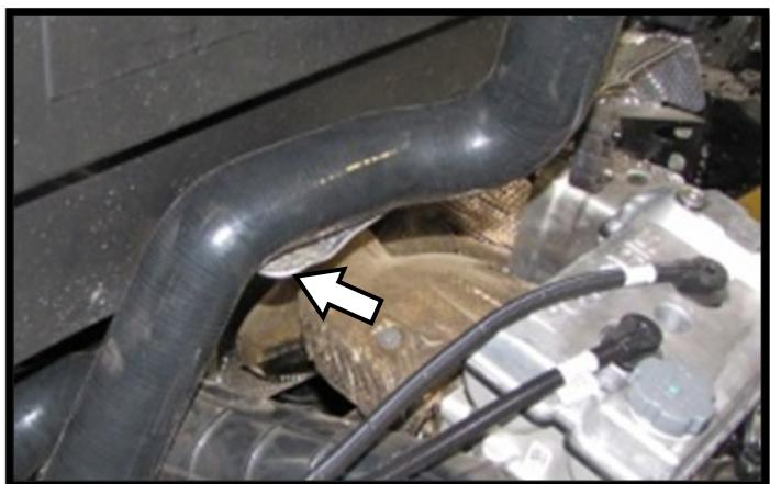
39. Next, slide the new air intake hose **75A** onto the air box inlet. Position it so that the high lifter logo is at the top of the hose and facing away from the cab when you reinstall the air box in the next step. Doing this before installing the air box will make the installation much easier and prevent having to adjust it. Attach and tighten down with hose clamp **HC40**.
