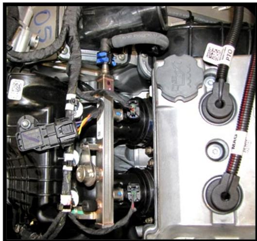
25. Remove the factory clutch housing inlet duct.
