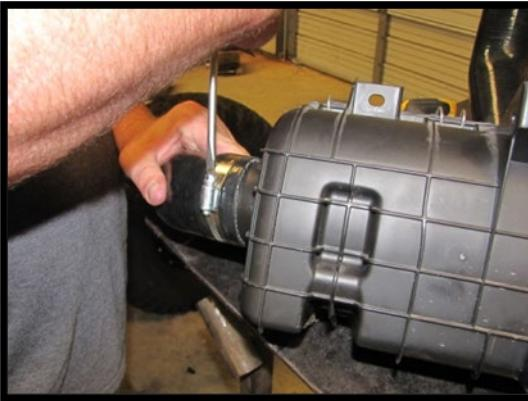
40. Reinstall the factory air box with the new air intake hose. The high lifter logo should be at the top of the hose and facing away from the cab.
