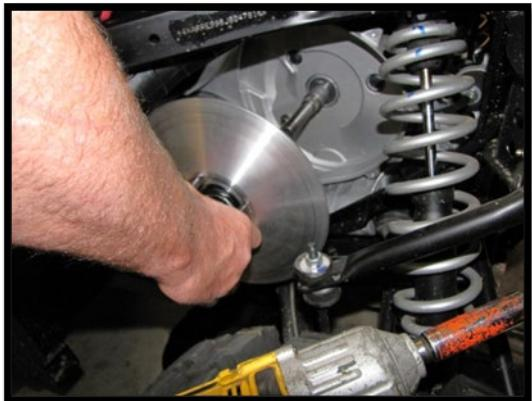
13. Remove the bolt and corresponding hardware from the primary clutch.
