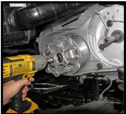
30. Reinstall the belt and secondary clutch
