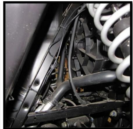
63. Find any precut holes or opening to route the vent line through to the front storage compartment. Once through, insert a barbed fitting **BHF-14-ST** into the vent hose, followed by a bellow **VB01**. Use **11" zip ties** to secure the hose and bellow in a place it won't get damaged.
