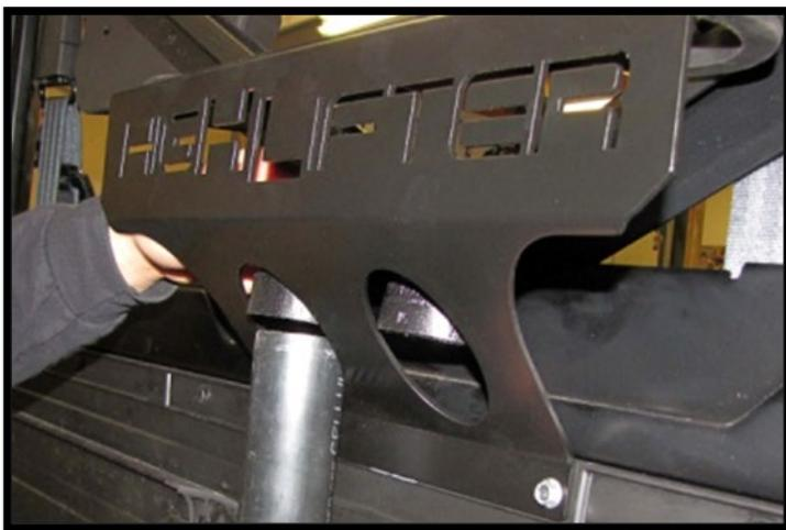
59. Once all final adjustments have been made. You need to attach and tighten the remaining hose clamps to the risers. Use a **HC40** for each 2" riser and a **HC36** for each 1 ½" riser.
