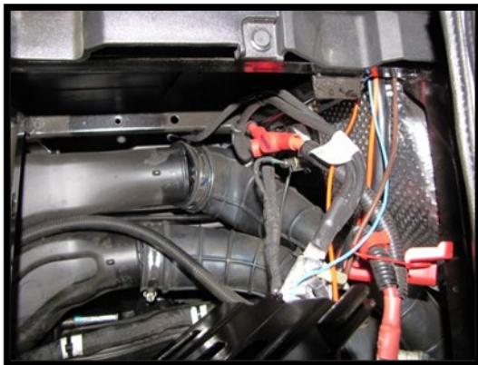
6. Now loosen the clamp from the air box inlet, and remove the factory air intake hose.
