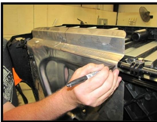
53. Trim the heat shield with a grinder where you marked it. Once finished, make sure it has proper clearance and trim extra if needed.
