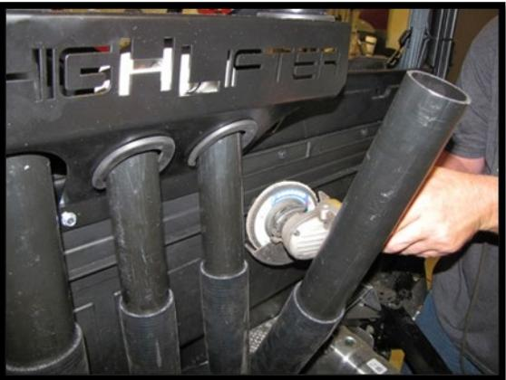
50. Slide the risers back into the riser plate. Then loosely attach the two **43R** riser caps to the top of the risers so that they sit flush to the riser plate. Do not fasten the hoses yet with clamps, you may need to make more adjustments in the following steps.
