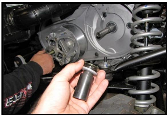
14. Use a clutch puller to remove the primary clutch.
