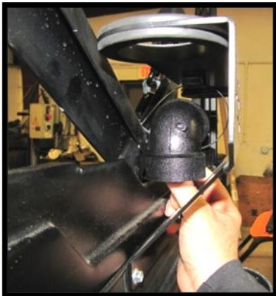
46. Slide two **SK-P-1527** (1 ½" x 10 ½" pipes) into the elbows. Then loosely slide the **RIGHT** riser into the corresponding clutch exhaust hose. Do not glue these into the elbows yet.
