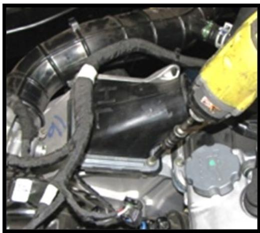
23. Also apply a generous amount of silicone under and around the edges of the port inside the clutch housing. This will help ensure no water will leak in.
