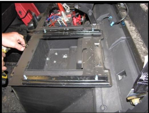
4. Under the passenger seat, lift and remove the storage box. Remove the battery and the battery support bracket. This will give you access to the factory intake hoses.
