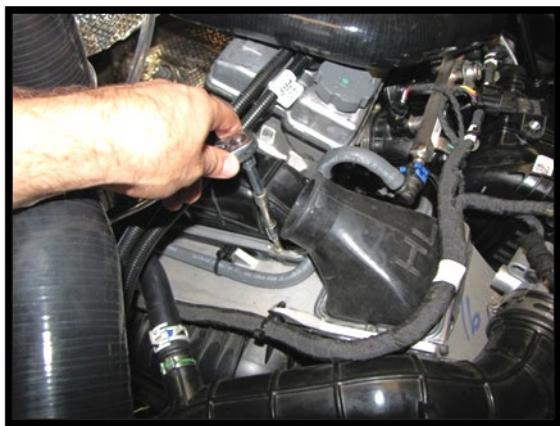
28. Next, use a clutch puller to reinstall the primary clutch.
