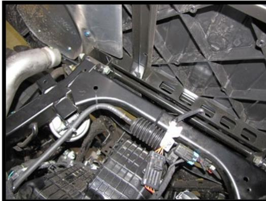
62. Find the front differential vent hose running up the frame on the front passenger side and disconnect it from frame. You will need the extra slack to reroute it up to the front storage compartment.
