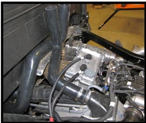
45. Connect and glue the 90 degree elbows **SK-EL-1501** and **SK-EL-1502** together. Then secure the elbows underneath the top of the riser plate with a heavy duty **18" zip tie** so that they are snug. This will keep them in place while you line up the risers in the next steps.
