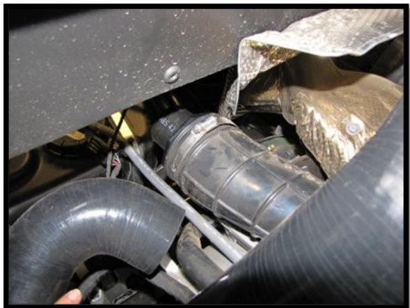
38. Insert the new clutch intake hose **75B** onto the pipe. Align the hose to the back of the cab and riser plate in the proper position. The high lifter logo should be at the top of the hose and facing away from the cab. Attach and tighten it with hose clamp **HC40**. You may need to bend the exhaust heat shield down at the edge to provide more clearance for the hose.
