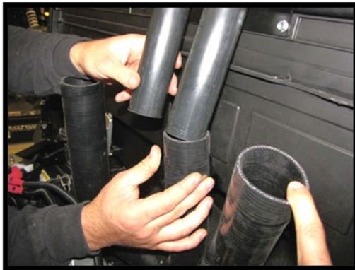
47. Loosely slide the small clutch exhaust hose **75D** onto the **LEFT** riser. **It is very important that it be positioned (as in the picture below) so that it can blow the excess engine heat out of the engine bay.** The high lifter logo should be at the top of the hose and facing away from the cab.
