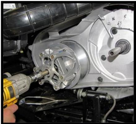
29. Use the factory bolt and corresponding hardware to complete the primary clutch installation.
