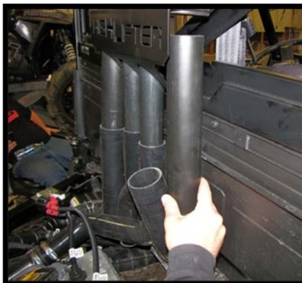
49. Once the 2" risers are lined up and you know where to trim, slide them out of the riser plate and pull them back. Use a grinder to trim the plastic lip so that each 2" riser can sit flush to the back of the cab.
