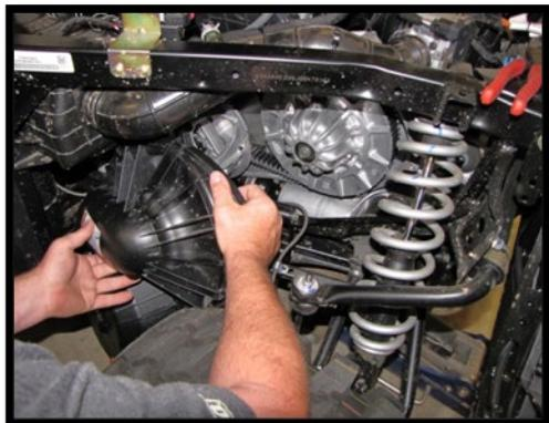
12. Remove the secondary clutch and the belt.
