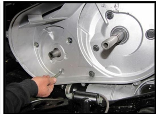
16. Before you can remove the four bolts from the right side of the clutch housing, you will need to remove the fuel rail and intake manifold first to be able to gain access to the nuts on the other side of the engine block. Process to the next step.
