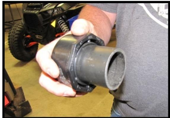
37. Insert the bushing adapter into the factory clutch intake hose and tighten the factory hose clamp.
