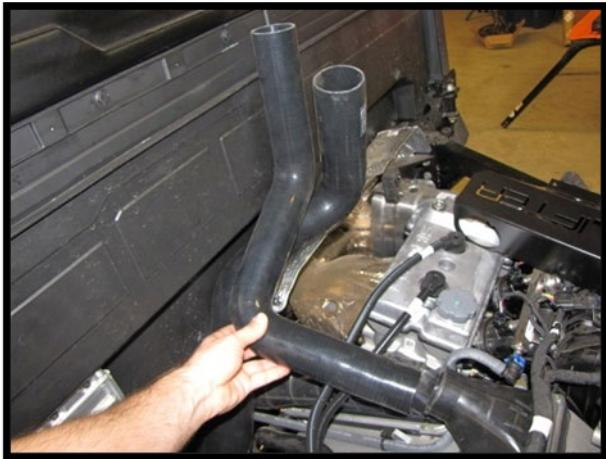
43. Once in the correct position, you may need to trim the excess hose that exceeds past the mouth of the clutch outlet duct.
