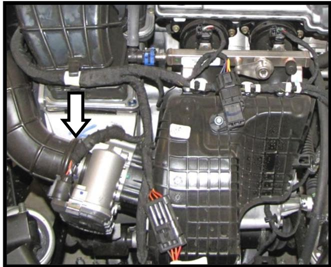
b. Tighten the two clamps around the throttle body adapter. Then insert and tighten the 8mm bolt and nut at the bottom back side of the intake manifold.
