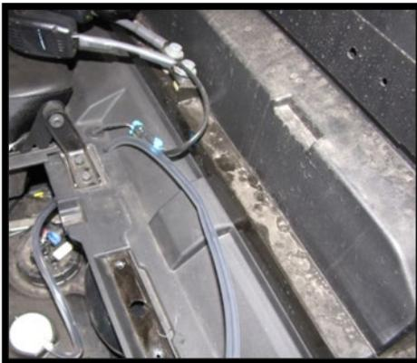
67. You can route the line through the cab frame behind the seats. If gas was to over flow from the vent line, it is necessary that it does not come in contact with the engine or exhaust. Use zip ties to secure it if needed.
