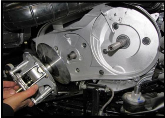
15. Remove the three bolts from the left side of the clutch housing. Apply silicone under the head of each bolt and then screw them back in.
