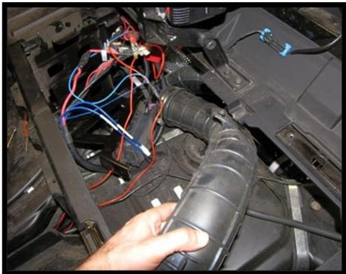
7. Next, loosen and remove the factory clutch intake hose. Also remove the adapter from the mouth of the clutch intake port fitting.
