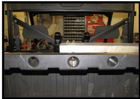
55. Using a reciprocating saw and a grinder, carefully trim the line you marked.
