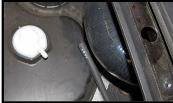
66. Insert the 5' vinyl hose **SK-VT-2** into the barbed fitting on the gas tank. You will need to route it up the cab. Drilling a routing hole in the plastic is optional. It just needs to be clear from being pinched or damaged.
