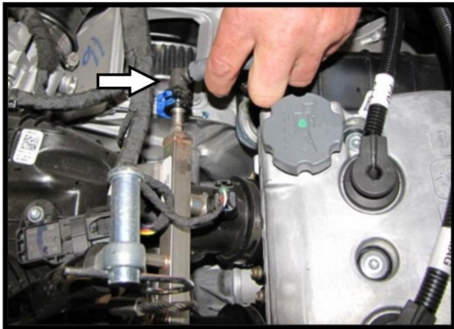
d. Reconnect the wire harness. Then re-secure the harness to the fuel rail with **three 8" zip ties**.
