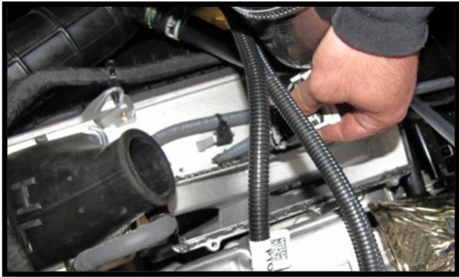
27. Before reinstalling the factory clutch inlet duct, you must insert all the factory screws back into the metal mount bracket and through the inlet duct. This will keep the duct in place when tightening the screws and reinstalling it. While installing, be careful not to pull the sides of the duct in. **This is necessary to prevent it from having an improper seal.** Once fastened, you will need to reach into the housing with your fingers and check for leaks or pulling of the edges.
