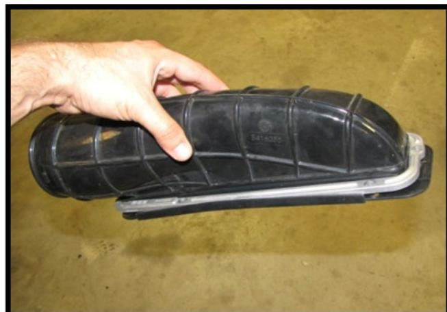
26. Apply a generous amount of silicone around the edge of the intake port where the duct makes contact.
