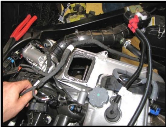
22. Slide the factory metal mount bracket onto the new **75N** clutch outlet duct. While installing, be careful not to pull the sides of the duct in. **This is necessary to prevent it from having an improper seal.** Once fastened, you will need to reach into the housing with your fingers and check for leaks or pulling of the edges.
