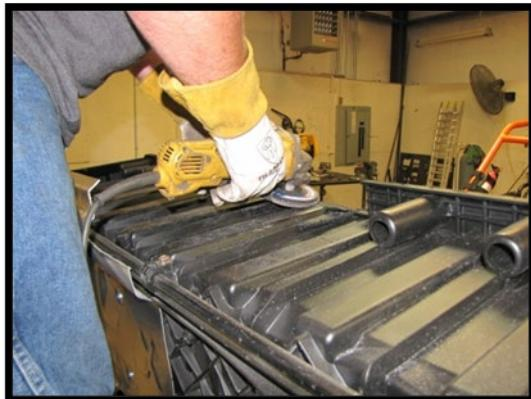
56. Gently fold the bed down to the snorkels to check clearance. Make adjustments, mark, and trim any extra plastic that's needed.
