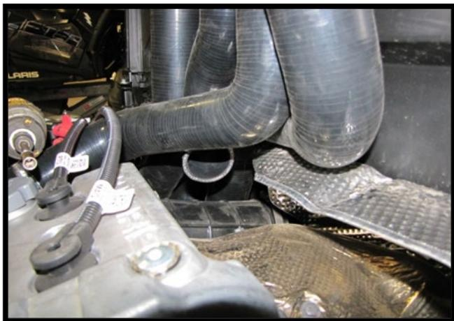
48. Loosely insert two **SK-P-223** (2 x 13 1/2" pipes) into the riser plate. You need to align them up so you can determine where to trim the plastic lip on the back of the cab in the next step.
